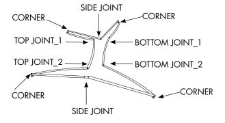
10' Frame (1) shown. 8' Unit has one less Bottom and Top Joint.
